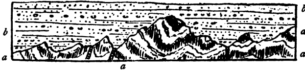
FIG. 1.—Ancient submerged Gneiss, aaaa , buried under Torridon Sandstone Grits and Conglomerates, bb .
